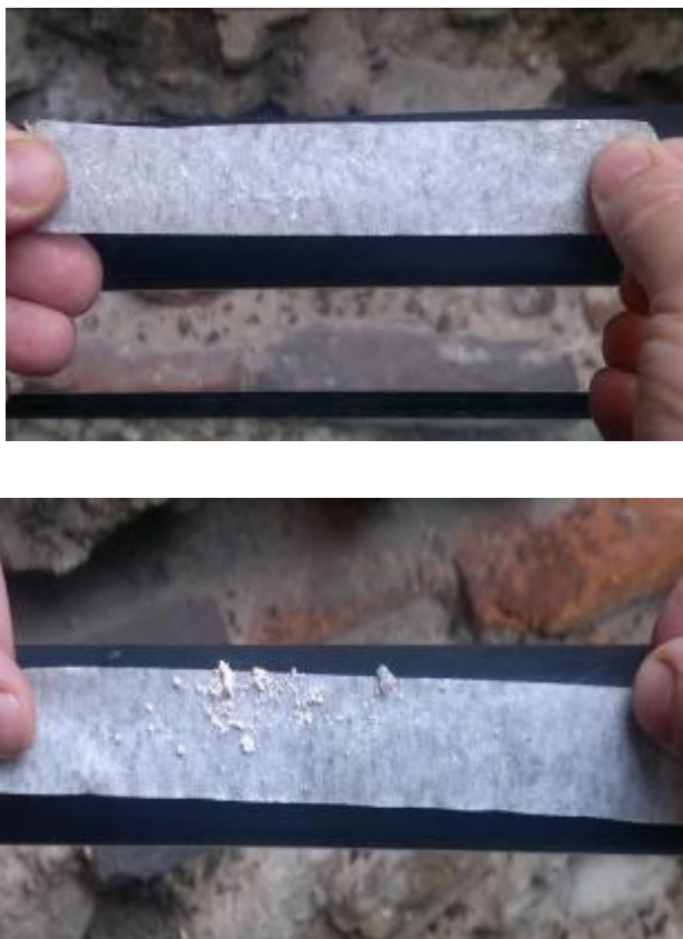
Figure 28 - Tape tests on chalk after HCT + OH100 treatment
