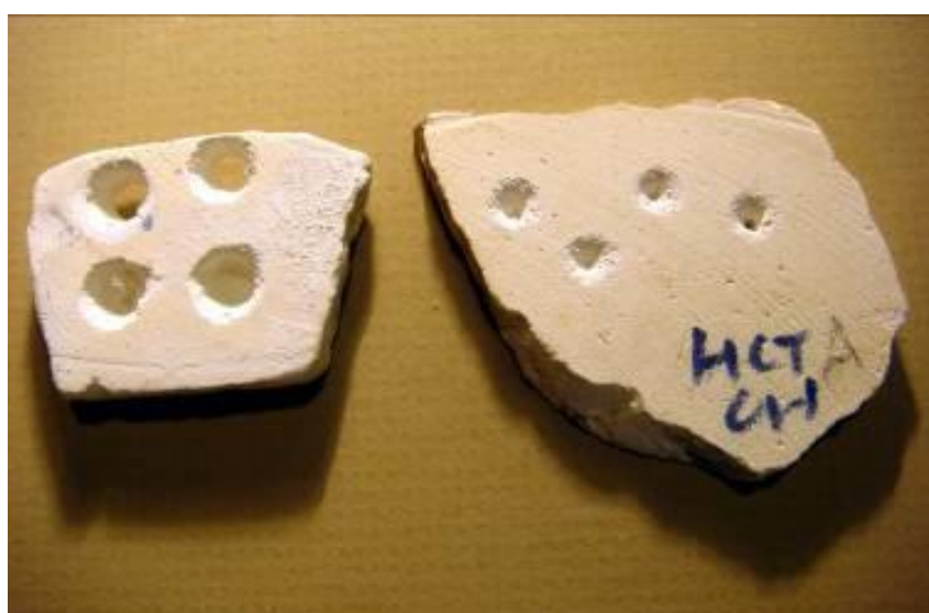
Figure 24 - Visual comparison of untreated control chalk specimen (left) and HCT +OH100 treated chalk sample (right) after micro-abrasion tests (courtesy of Irving Slavid, MCC )
