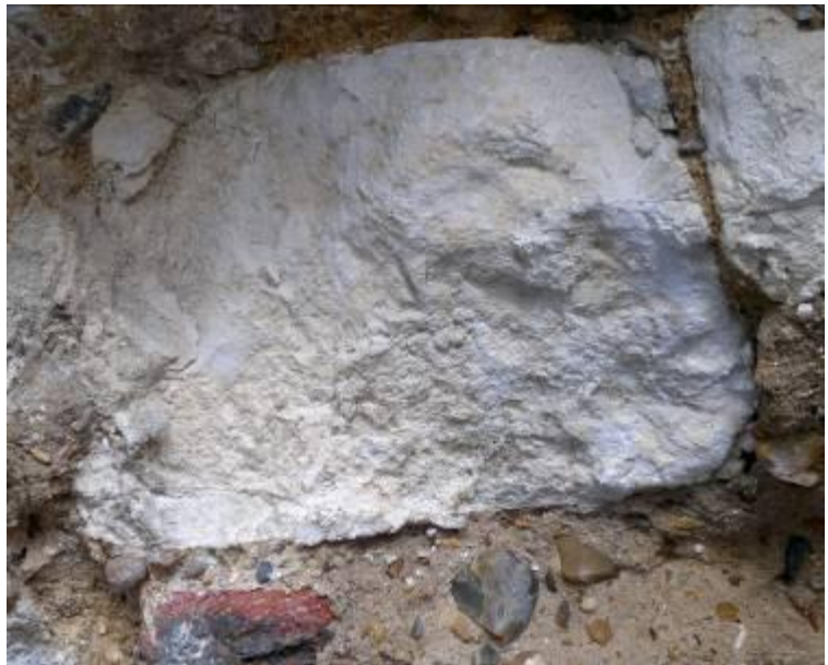
Figure 23 - Nanolime deposits ('bloom') to substrate surface associated with solvent evaporation/penetration failure
